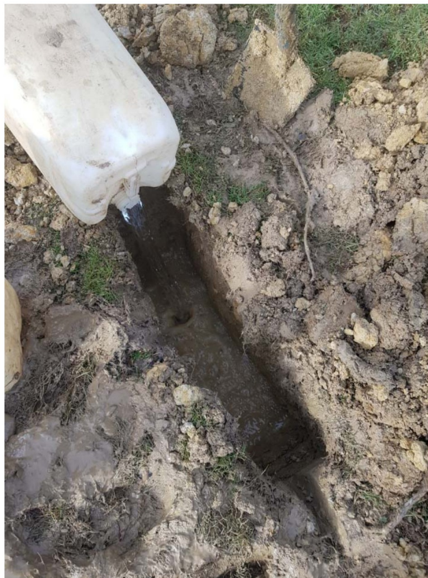
Photo 3. Preliminary BRE365 infiltration test – indicating clay soils
