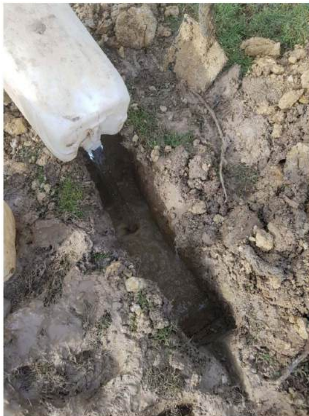
Photo 3. Preliminary BRE365 infiltration test – indicating clay soils
