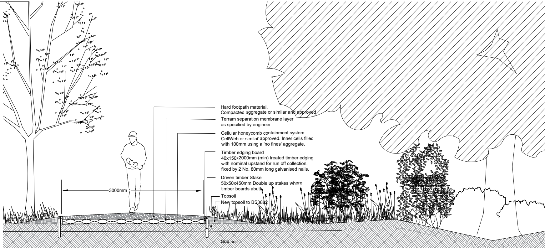
Section EE - within root protection area
