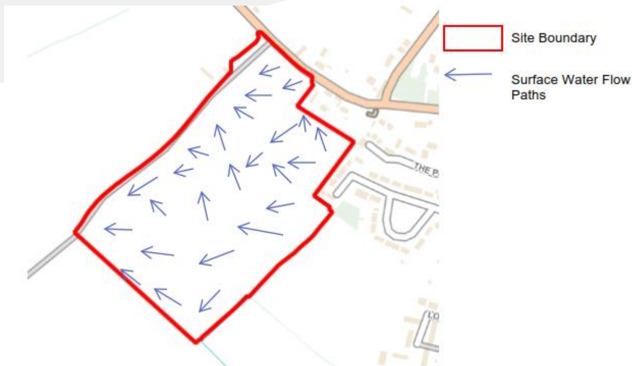
Figure 3.1: Existing surface water flow paths
