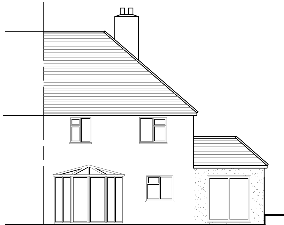
Proposed Rear Elevation 1/100
