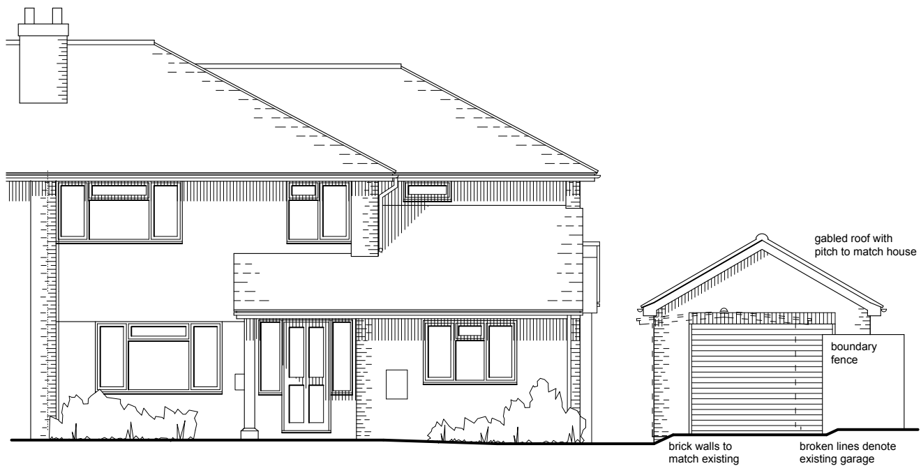
North West Elevation
