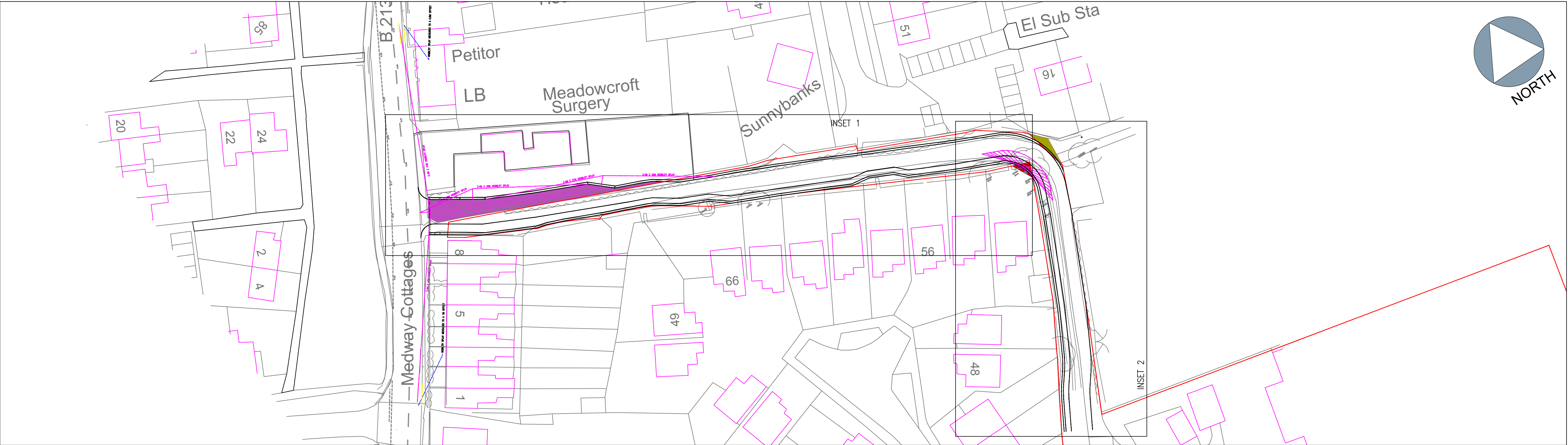
GENERAL ARRANGEMENT – SITE ACCESS ROAD (SCALE 1:500)
