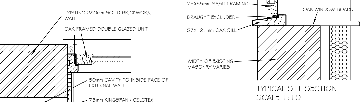
PLAN OF JAMB TO MAIN BARN OPENING SCALE 1:10
