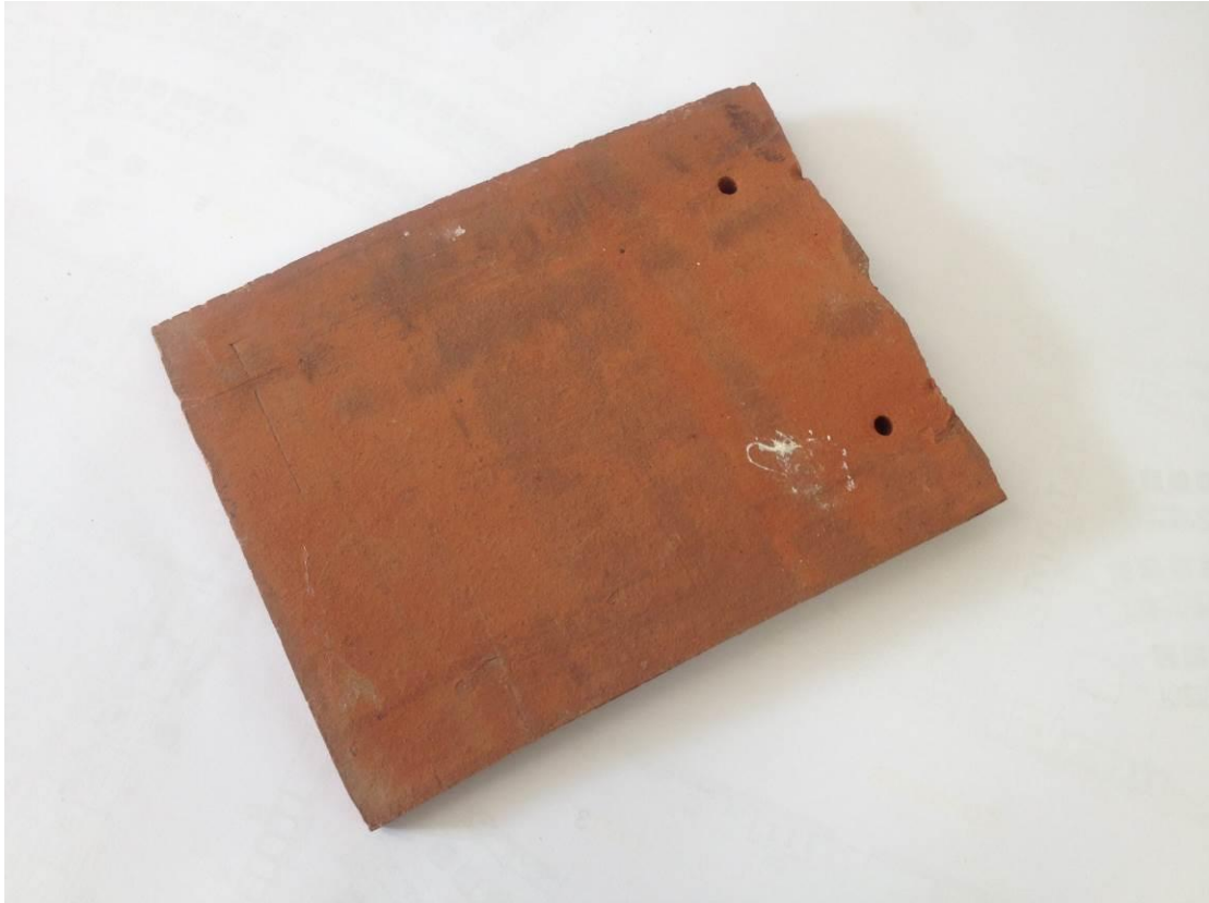
1.3 – Roof Tile; Marley Acme double camber clay roof tile 'burnt flame' [top side]
