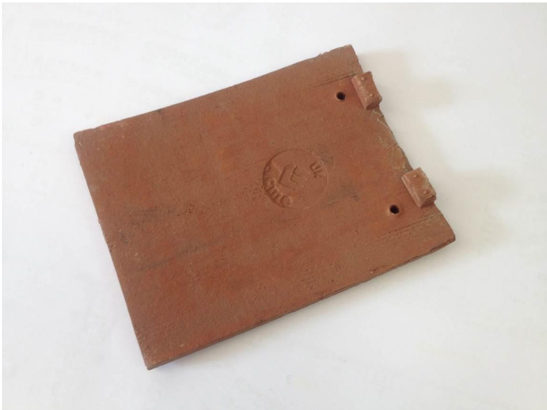
1.4 – Roof Tile; Marley Acme double camber clay roof tile 'burnt flame' [underside]
