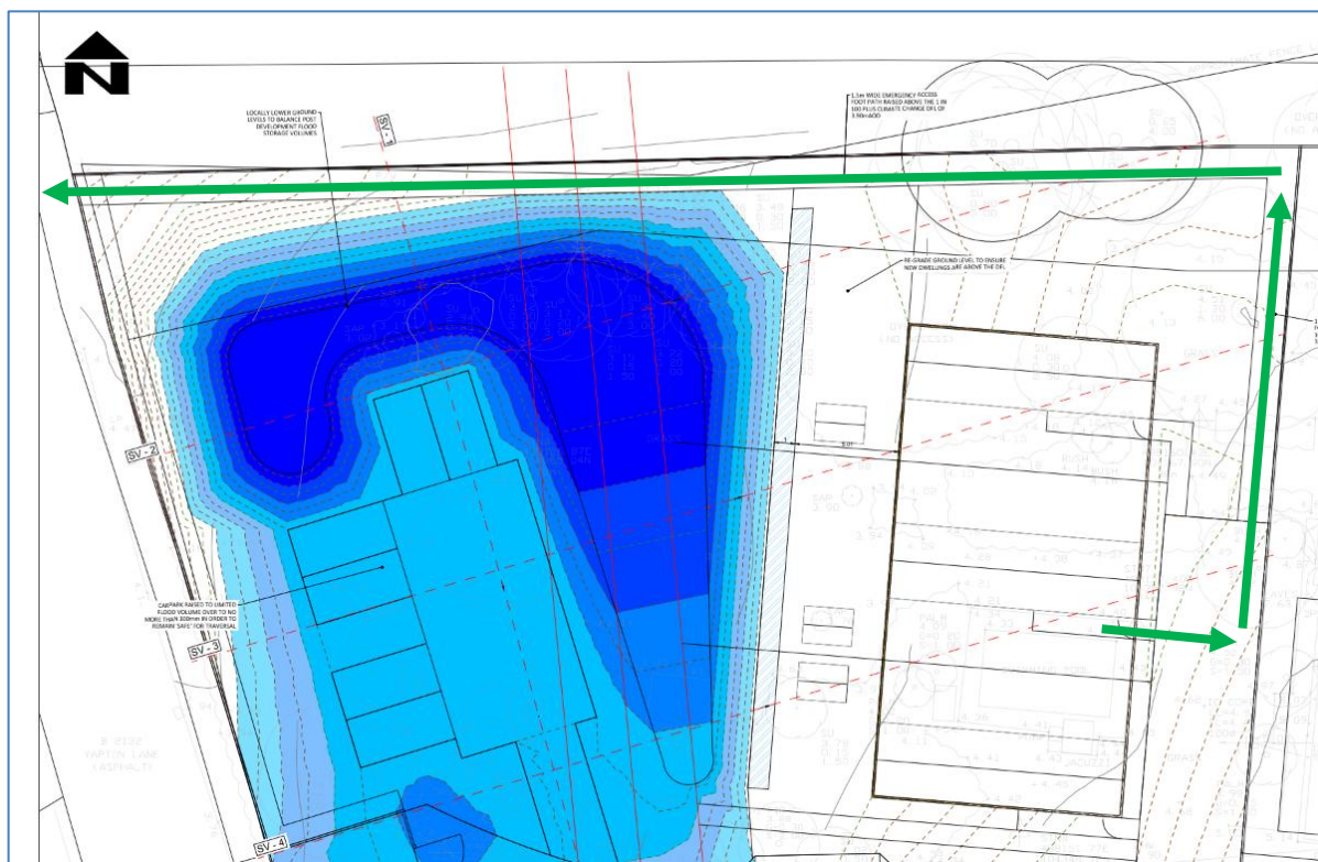
Figure 11 – showing surface water flood extents in the DFE, and the proposed access/egress route away from the static caravans onto North End Road.
