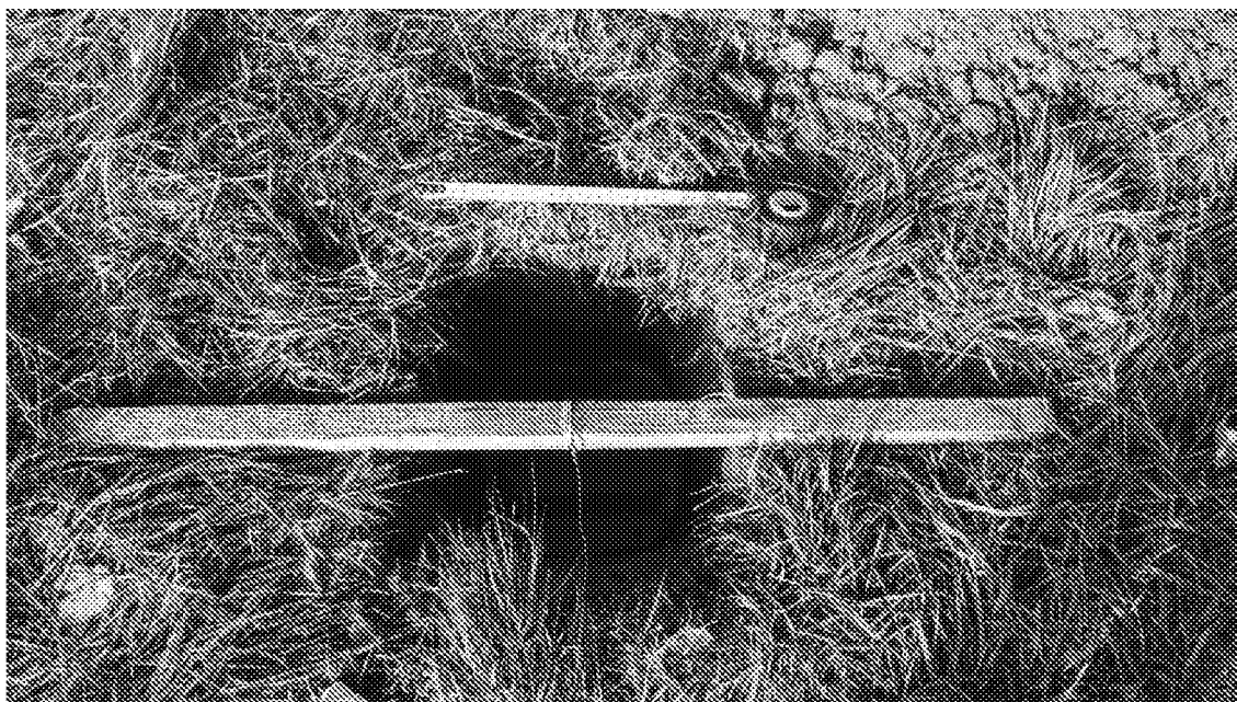
Figure 15 Spoil from hand pit 03 grading from slightly gravelly very silty fine sand to clayey silt with rare flint gravel (left to right).
