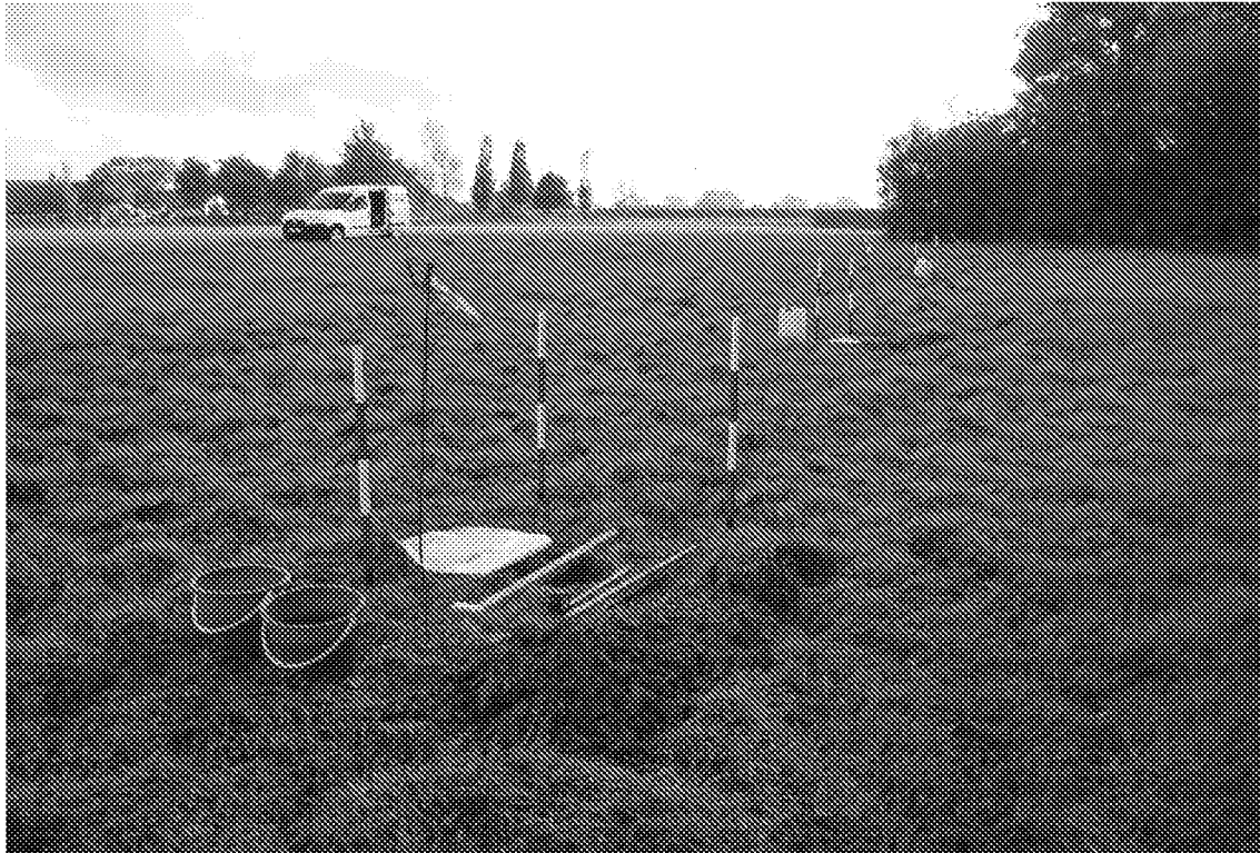
Figure 4 View of completed hand pits facing south with suspended level loggers (HP03 near, HP01 furthest).
