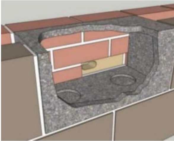
Figure 8. A schematic of how the Cambridge full-face swift brick leads into a cavity created by the prior installation of the Swift maxi nesting box.
