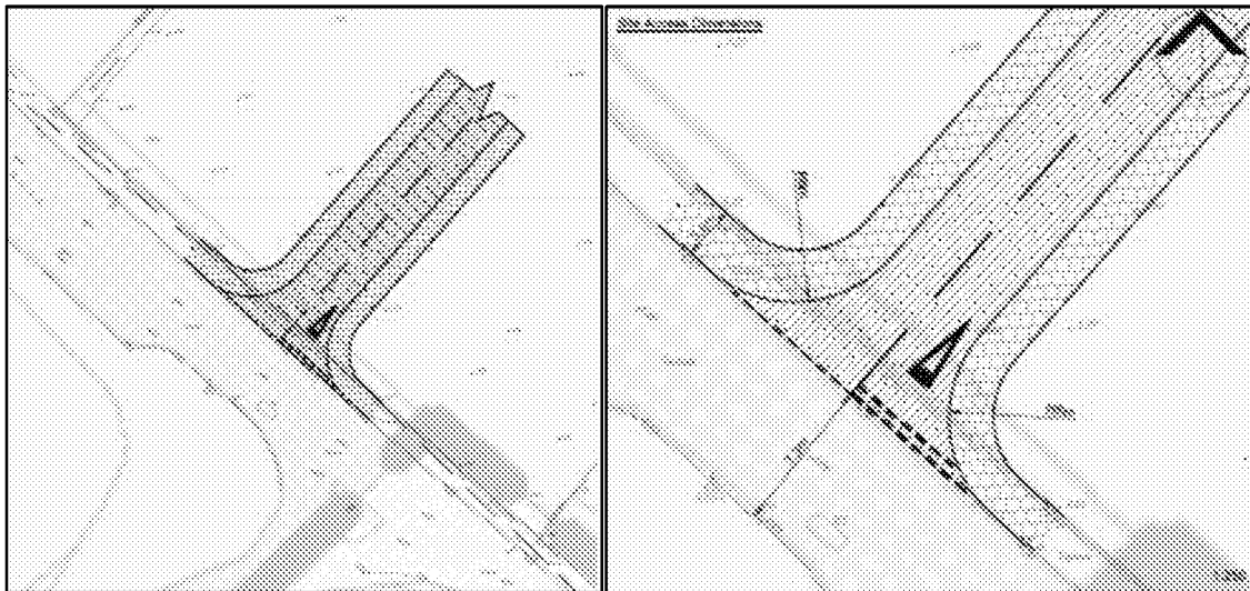
Figure 4.2 Site Access Arrangement
