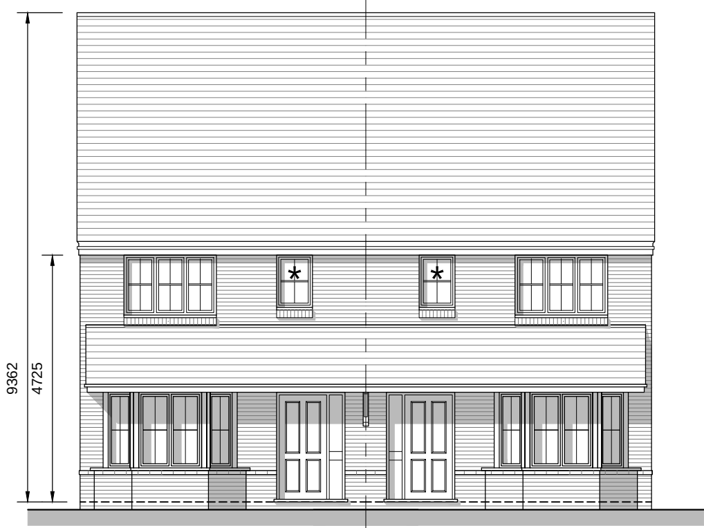
Front Elevation * - Obscured glazing Plots: 71 - 72
