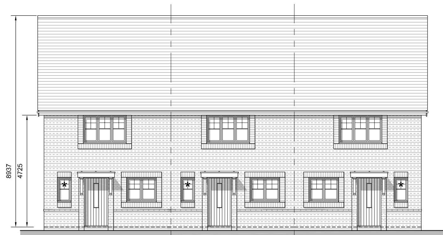
Front Elevation Plots : 182/183/184, painted brick
