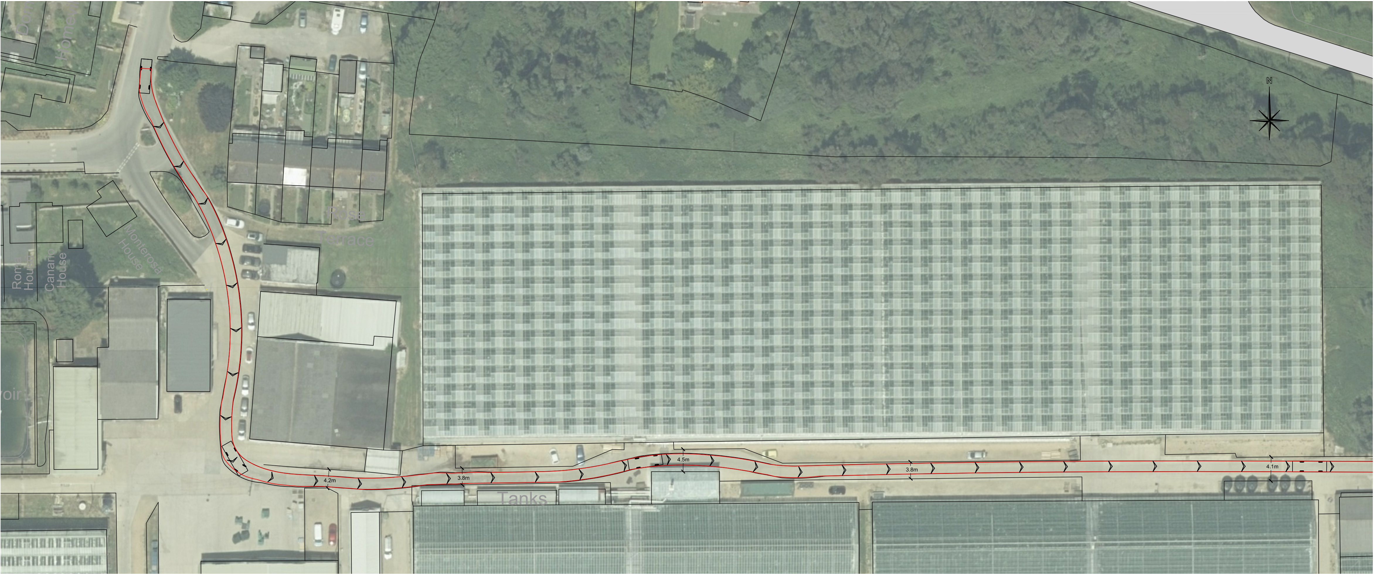
Fire Engine Swept Path - Part 1
