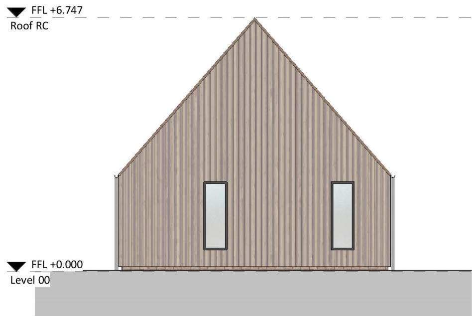
④ West Elevation - Remembrance Court 1 : 100
