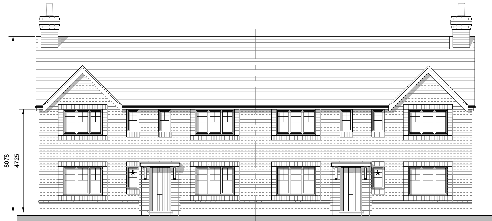
Front Elevation Plots : 148/149, painted brick
