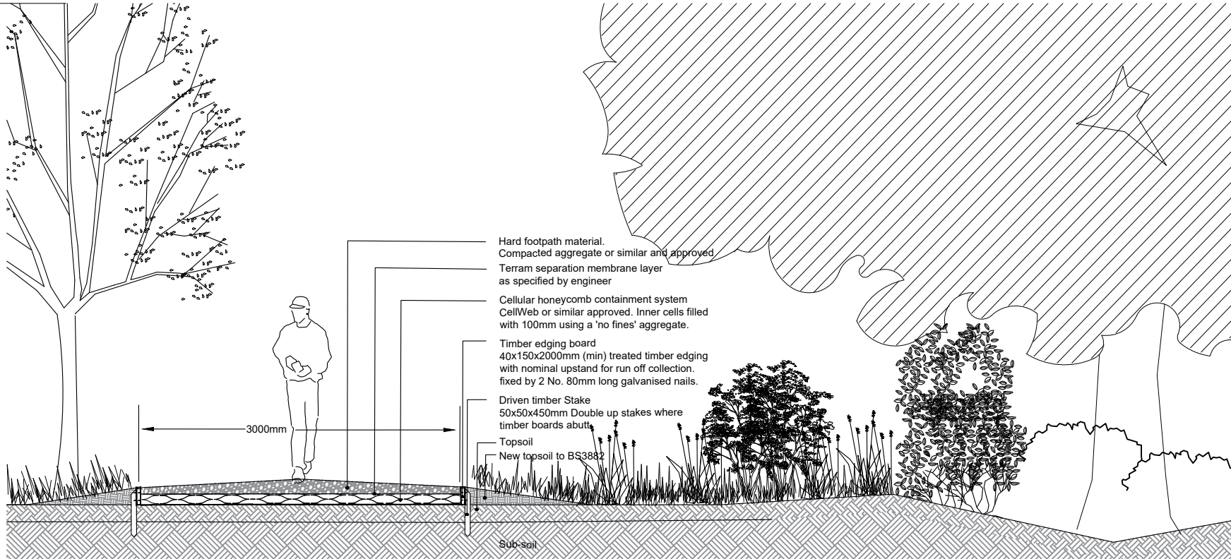
Section EE - within root protection area
