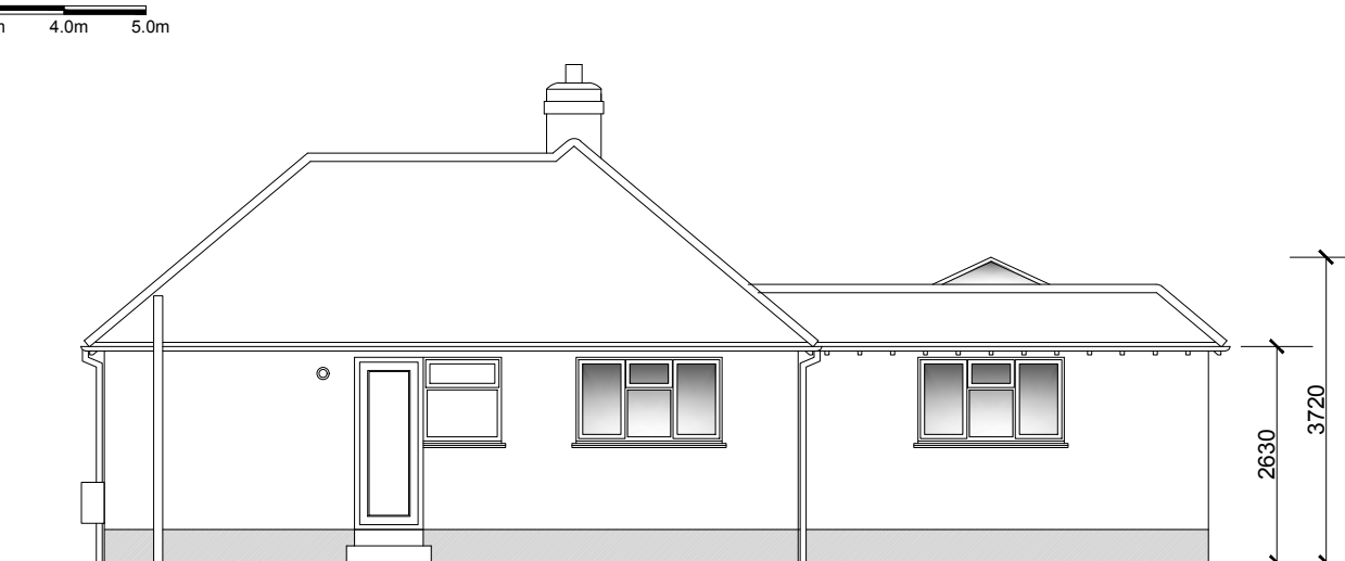
Proposed West Elevation (side) 1:100 @ A1
