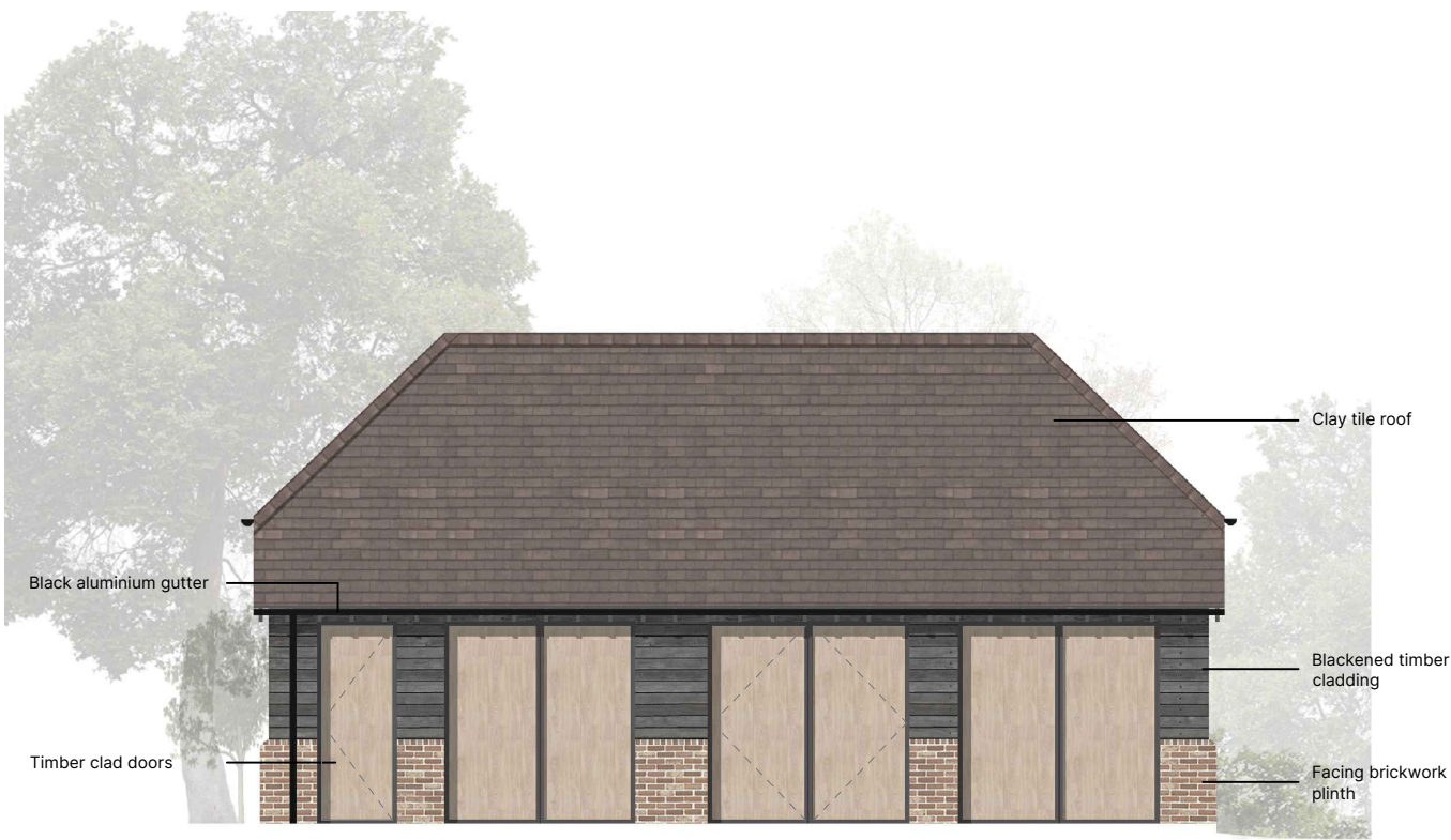
WORKSHOP - NORTH ELEVATION [Front] 1:100
