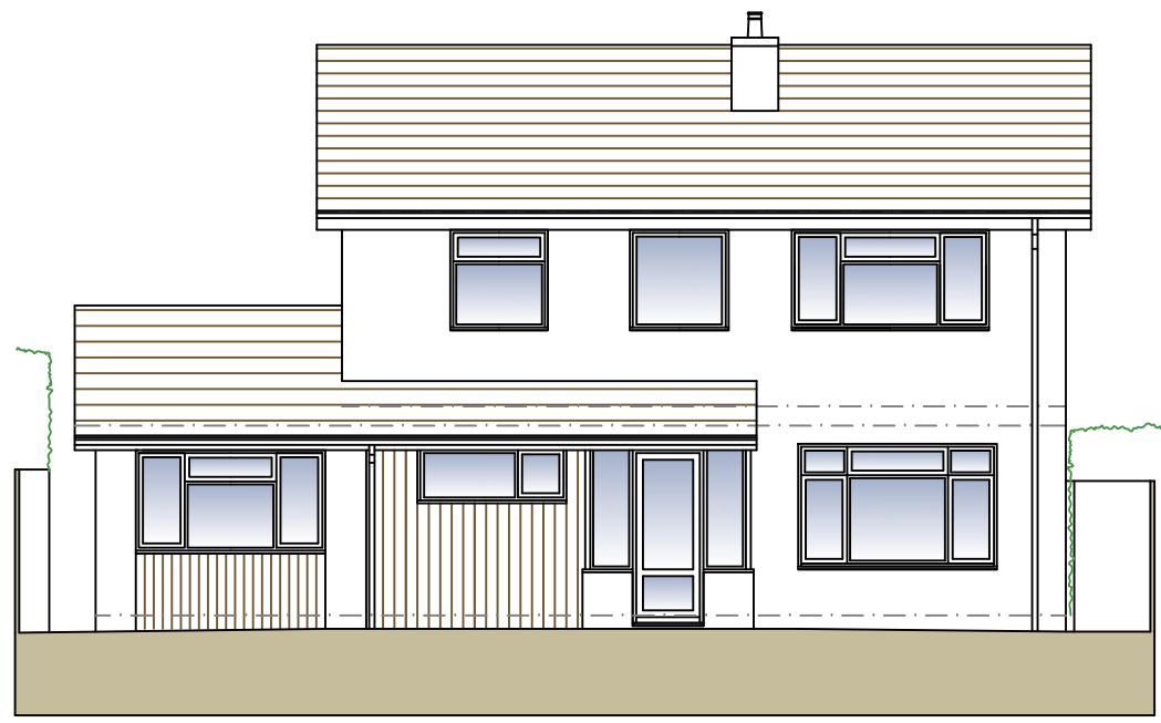
Existing North (Front) Elevation 1:100
