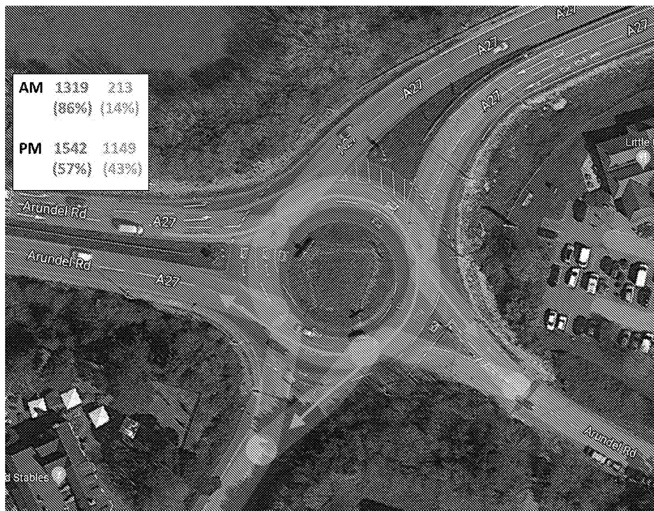
Figure 3 Fontwell West Roundabout West Approach Lane Usage
