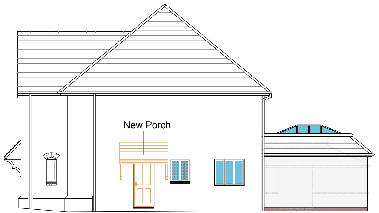
South Elevation – (Side) 1:100
