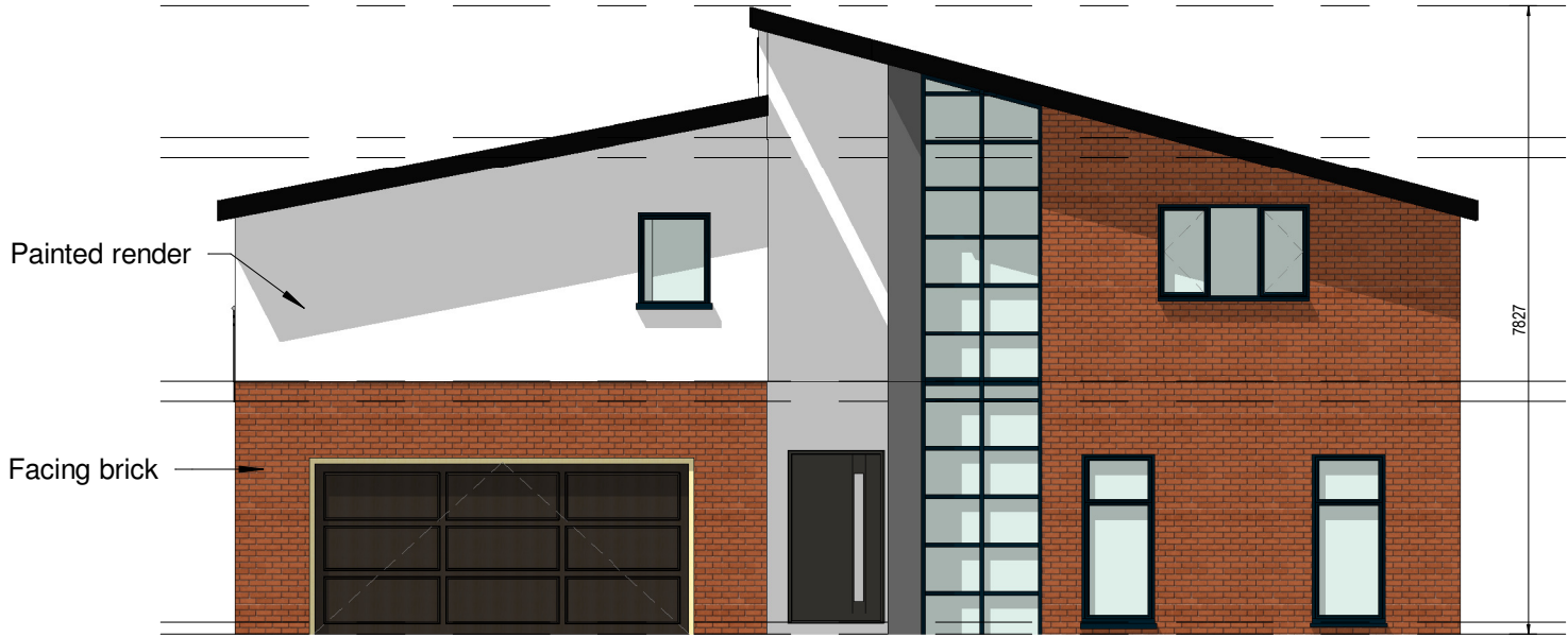
2 PR_01. Building-B. Front Elevation 1 : 100
