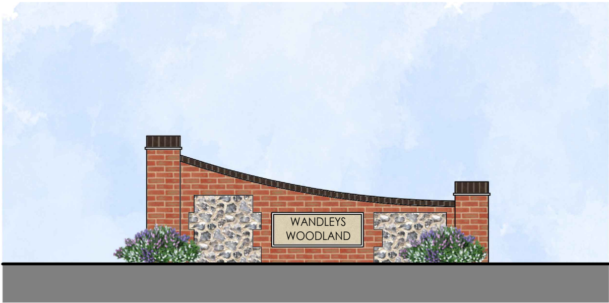
Entrance Feature Wall Elevation 1:50
