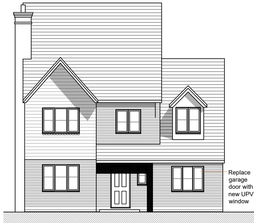
FRONT ELEVATION [south-west] 1:100
