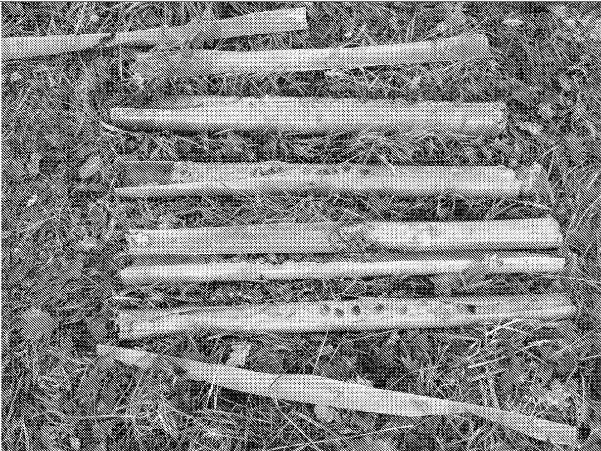
PLATE 4 – Cores from Window Sample borehole WS4
