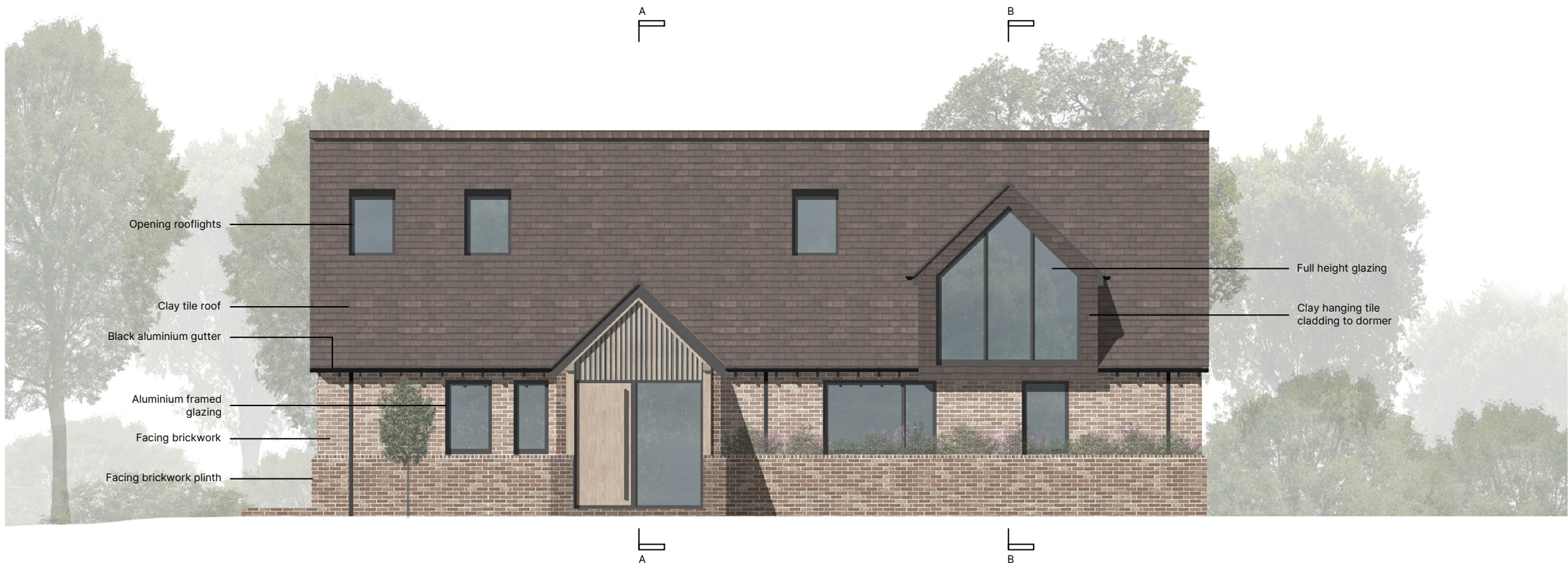
EAST ELEVATION [Front] 1:100
