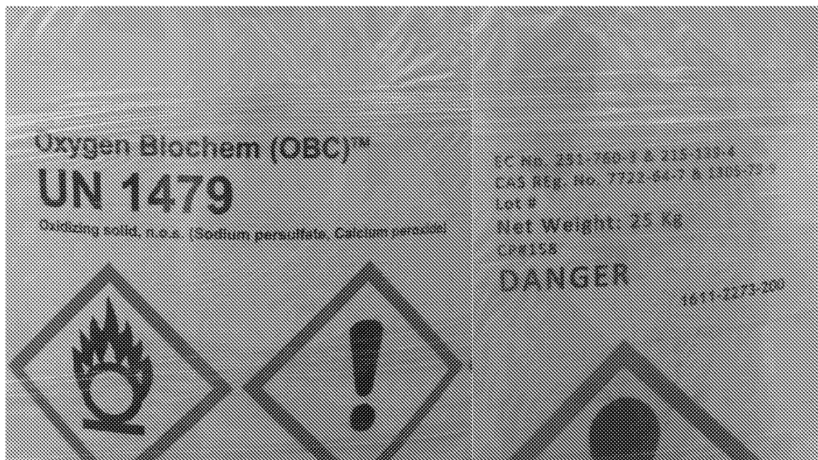
Figure 11 - Detail of oxidising agent specification as displayed on the packaging. OBC was stored in sealed 25kg tubs in a specially designated area of the site.
