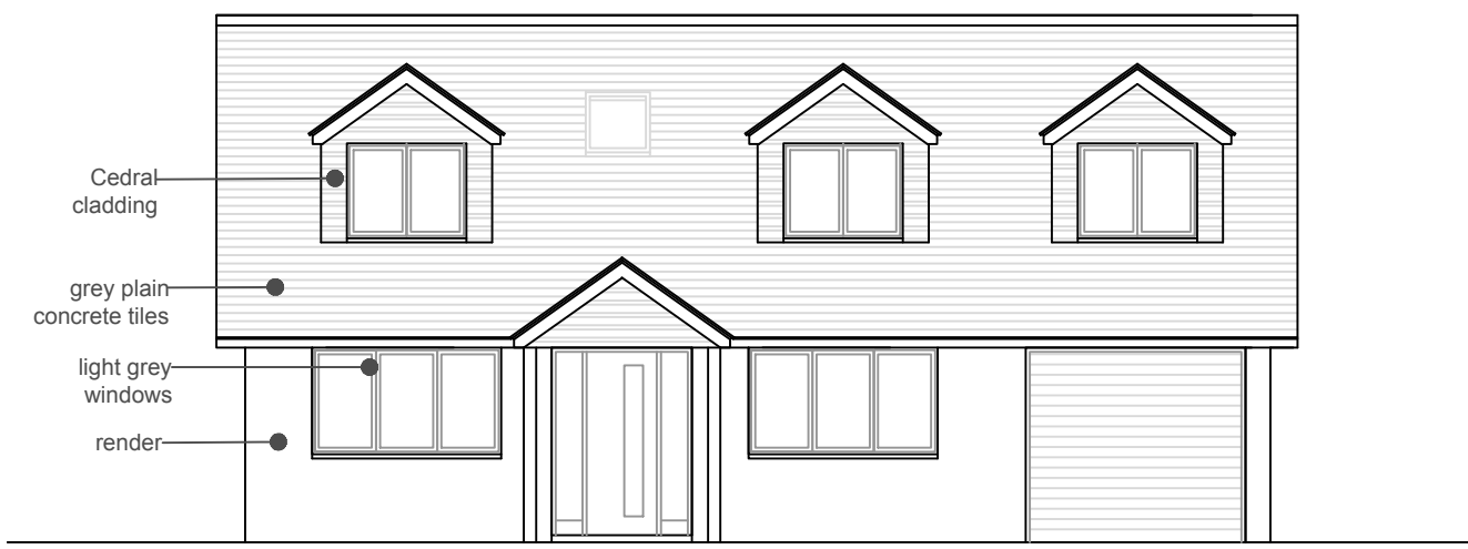
Front Elevation (north)
