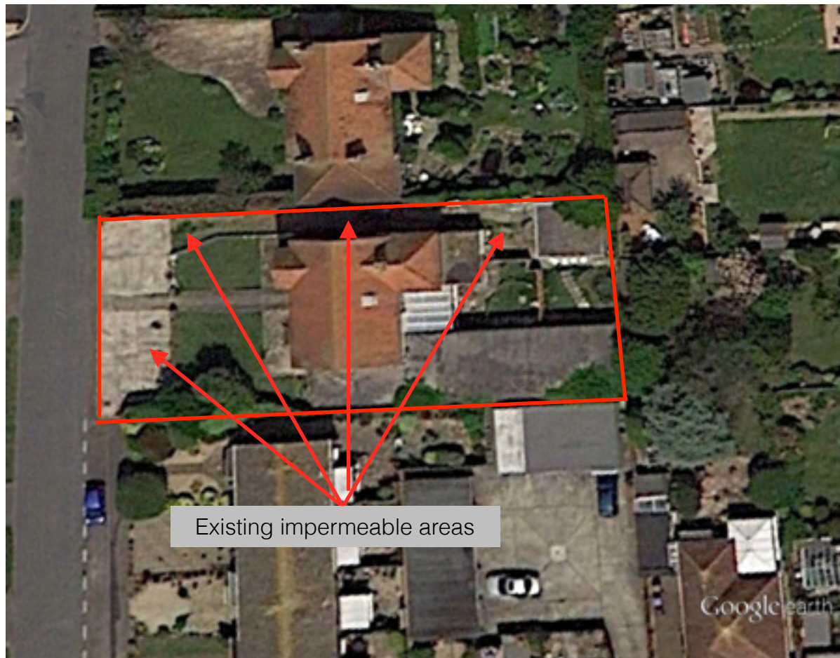
Fig 1. Existing site layout
