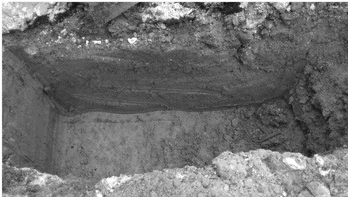
Plate 1: Excavated trial pit (SA401) showing Made Ground overlying River Terrace Deposits.
