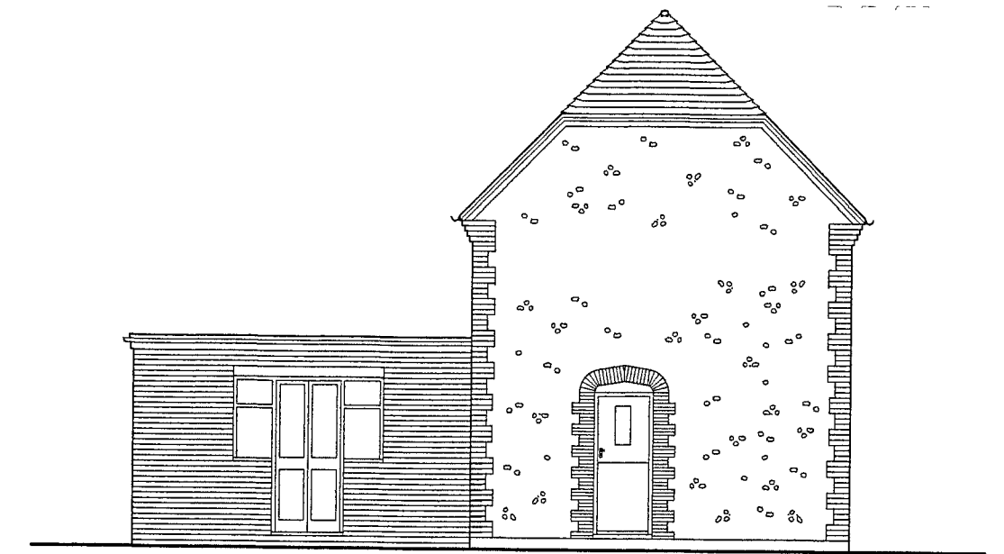
East Side Elevation - as existing
