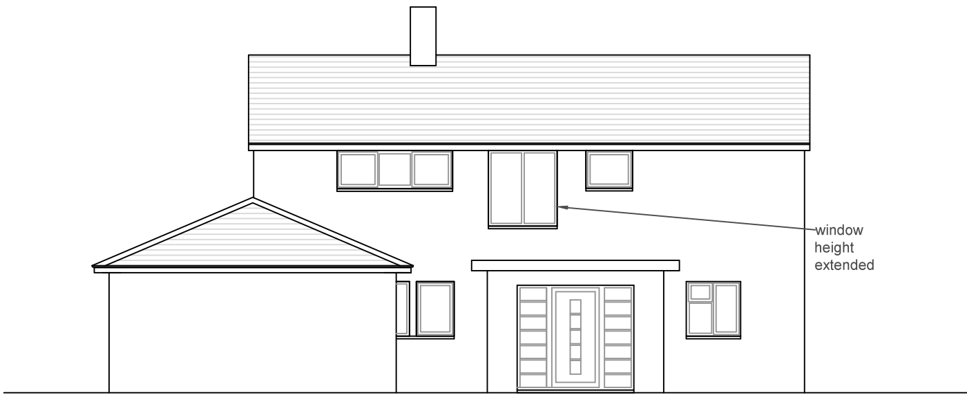
Front Elevation (north)
