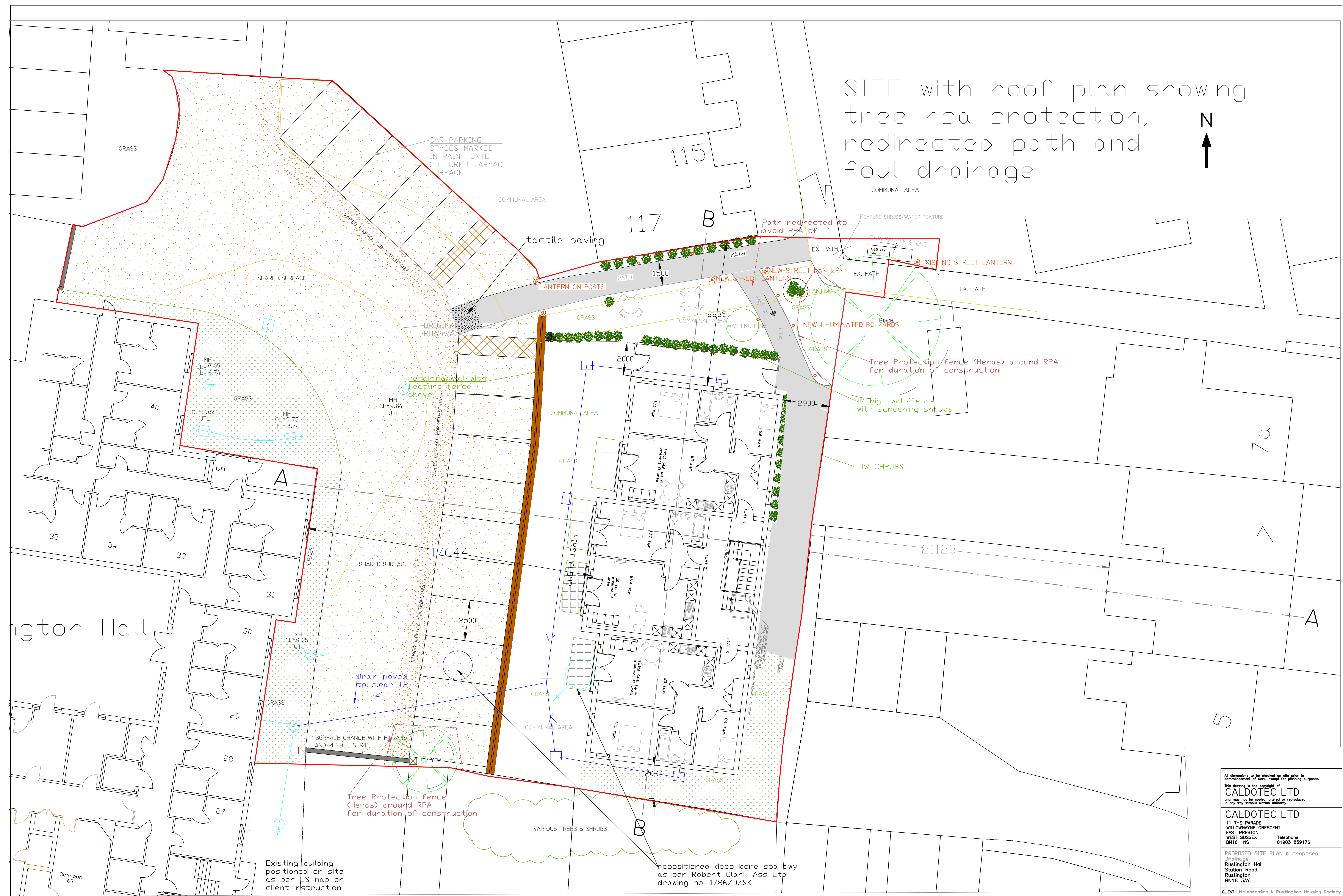
SITE PLAN showing proposed drainage 1:100
