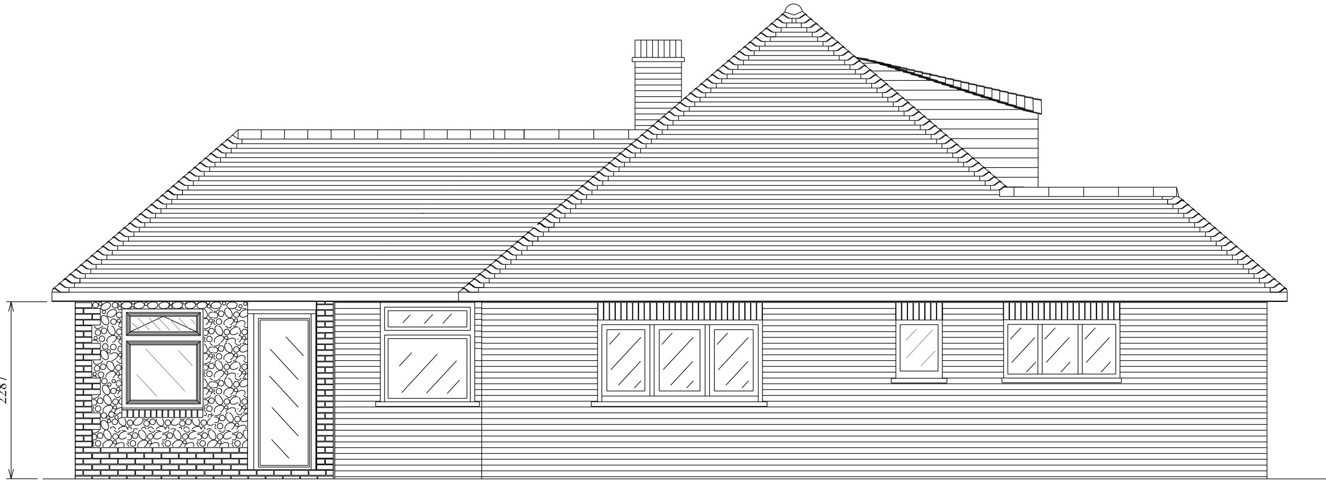
EXISTING SIDE ELEVATION (East) (Scale 1:50)
