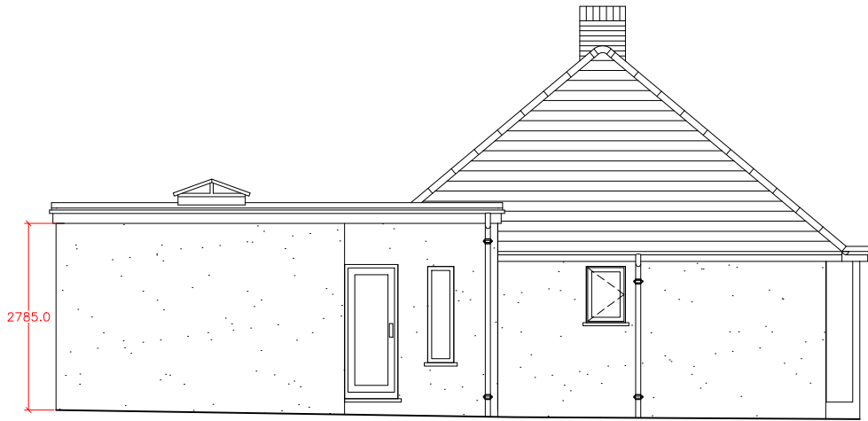
Side Elevation (North-West Facing) (Scale 1:100)
