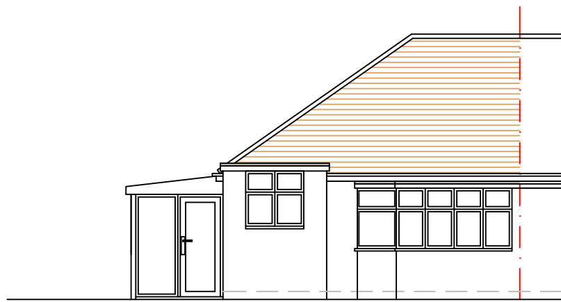
Existing Rear Elevation (East). Scale 1:100
