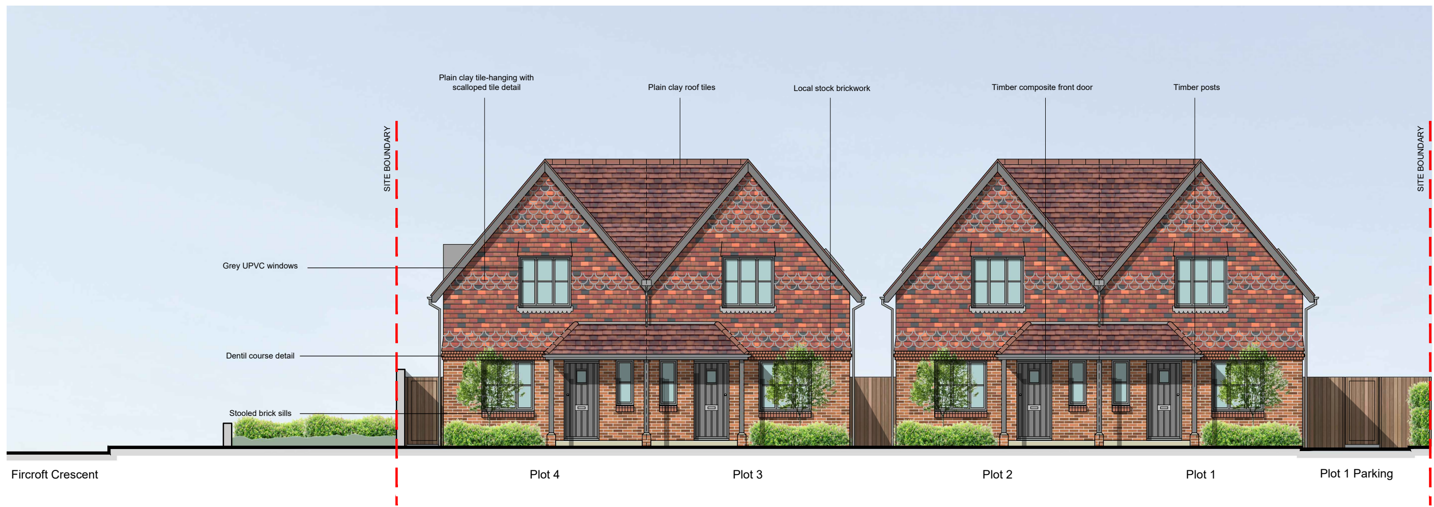
FRONT (NORTH) ELEVATION 1:100
