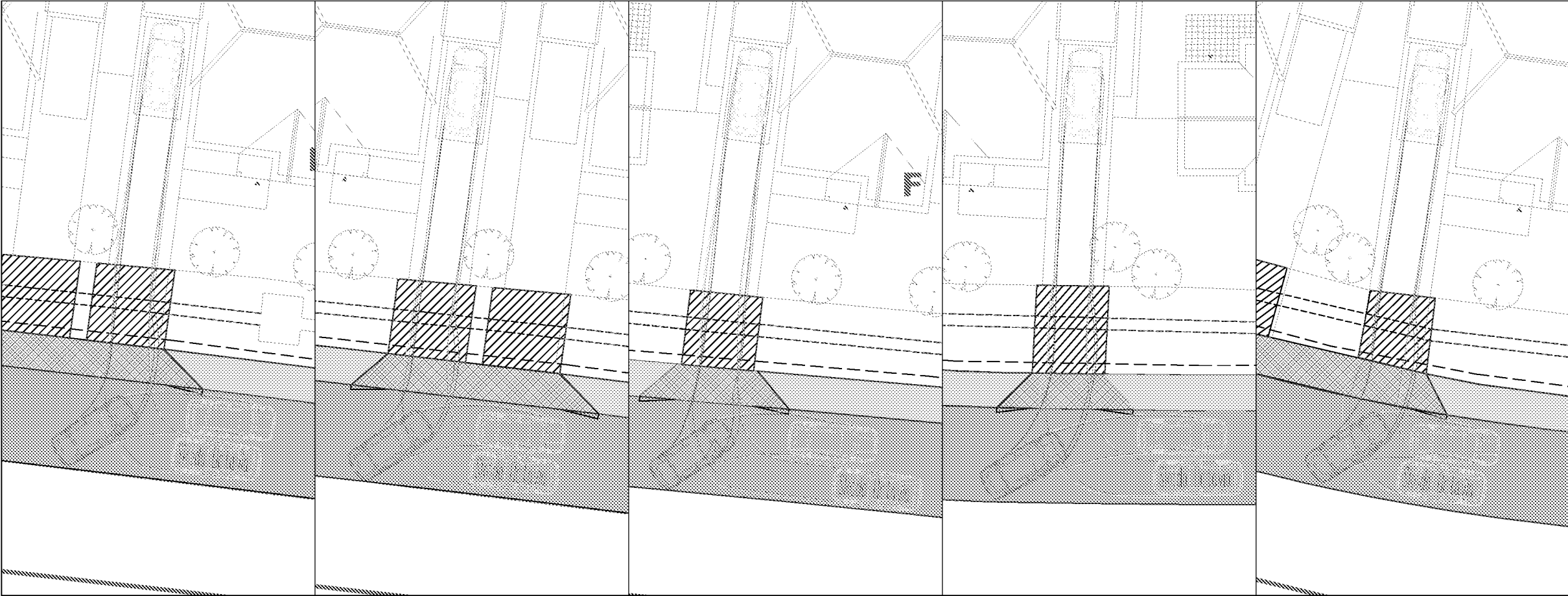
UNITS 47, 48, 49, 76 AND 77 DRIVEWAY ACCESS TRACKING (SCALE 1:250)
