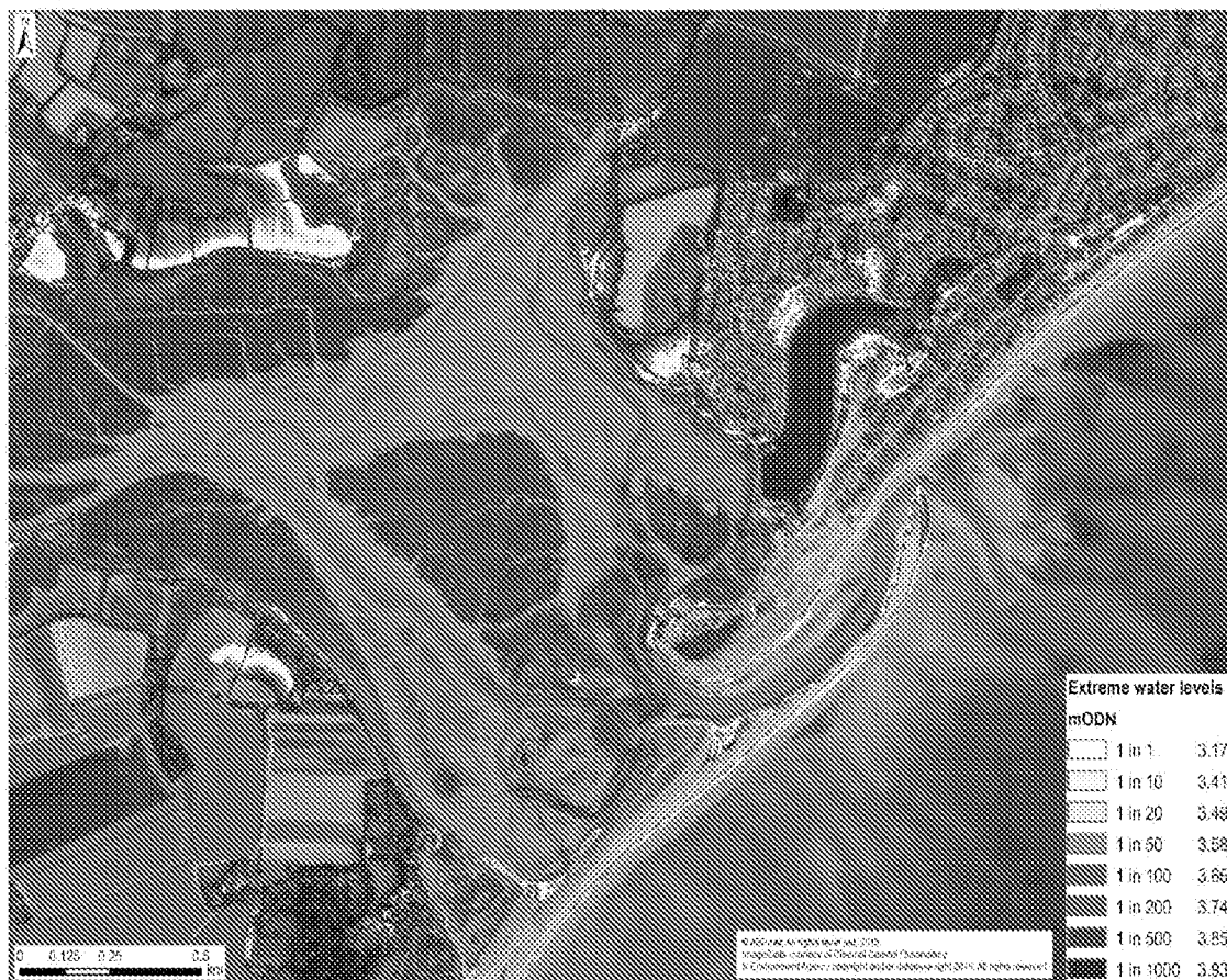
Image 12. Land elevations around Pagham Harbour equating to projected extreme water levels
