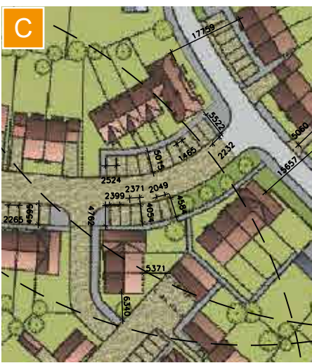
Analysis reveals sub-standard size of parking spaces, as well as sub-standard garden sizes. These will need to be adjusted to meet Arun's standards.
