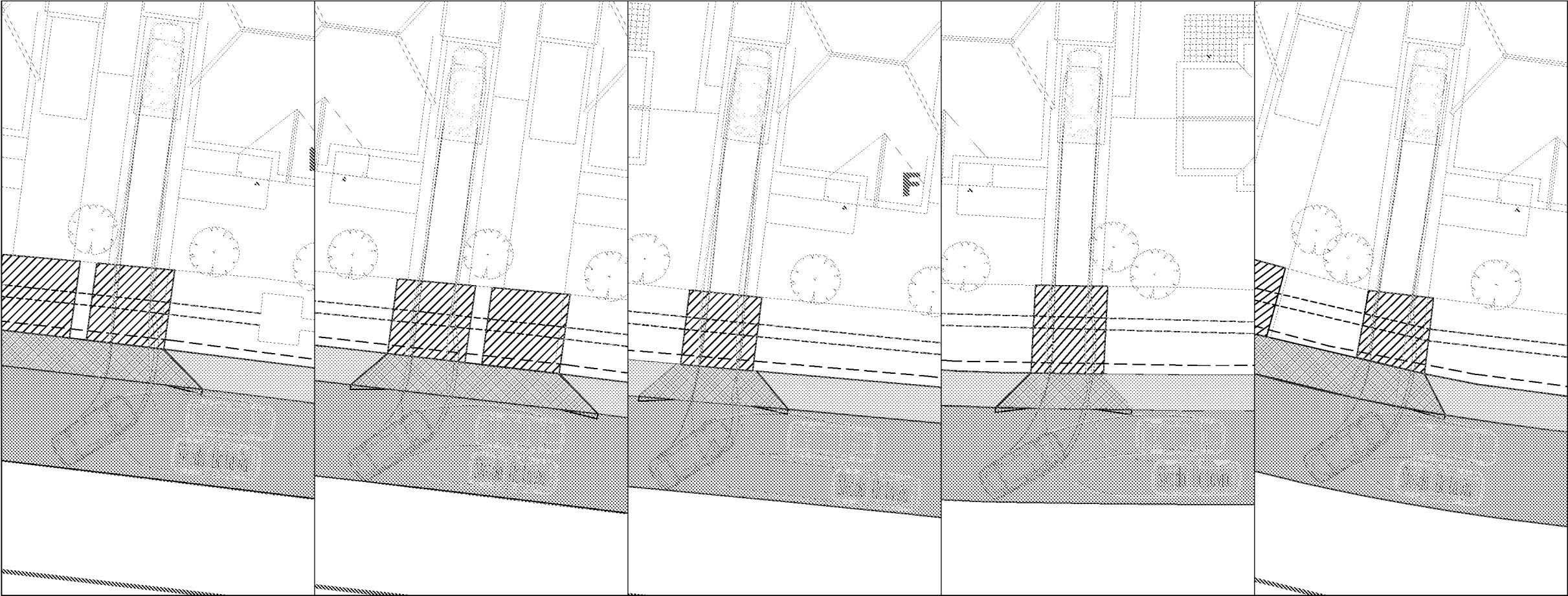
UNITS 47, 48, 49, 76 AND 77 DRIVEWAY ACCESS TRACKING (SCALE 1:250)
