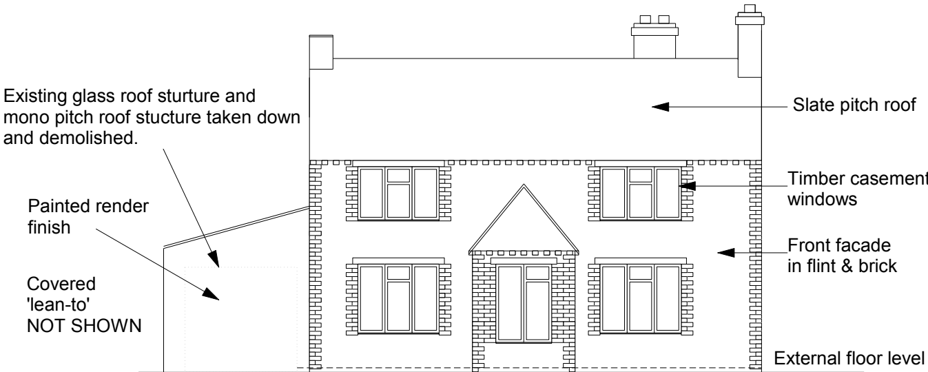
Front Elevation Existing (South) Scale 1:100
