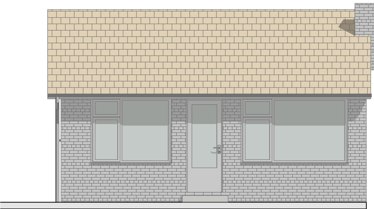
Existing East/Rear Elevation 1:50
