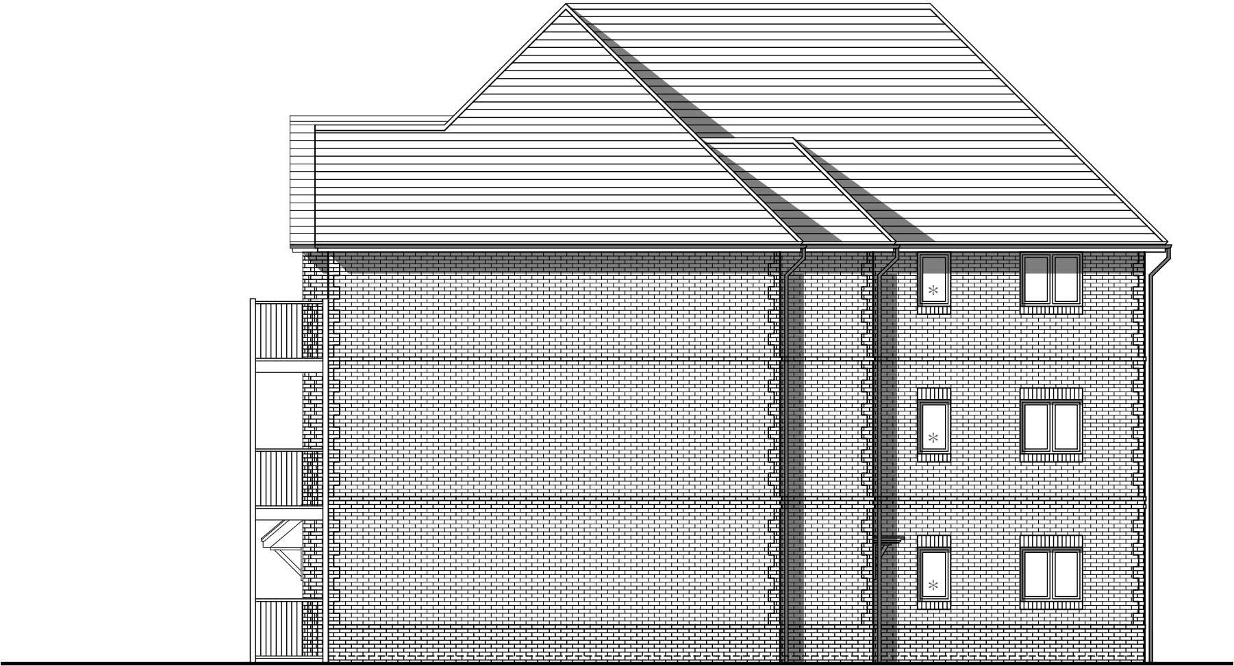
SIDE ELEVATION * OBSCURED GLAZING
