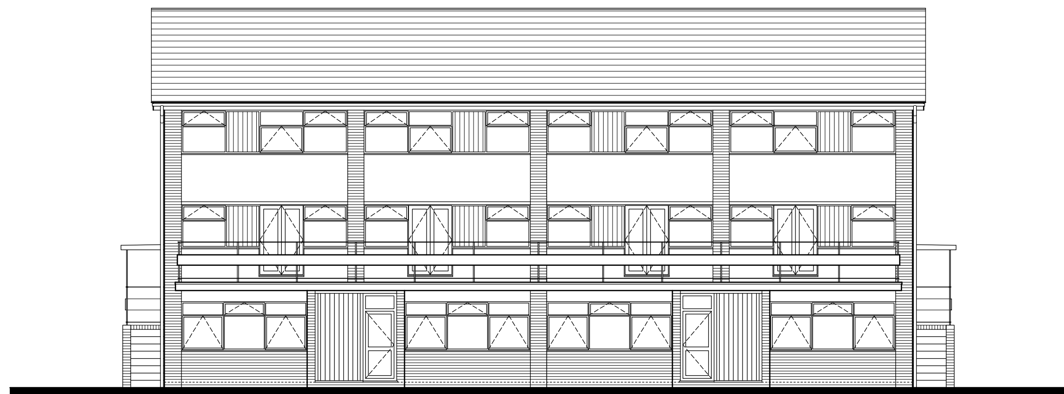
6 Dwelling Block. Numbers 1-6 Front Elevation. Scale 1:100.
