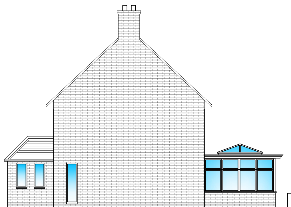
EXISTING SOUTH ELEVATION 1:100
