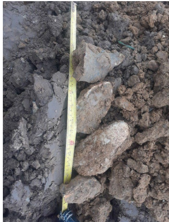
6/Pit subsoil stone
